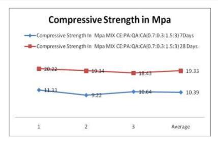
Cement 35% Replaced by Pond Ash and Sand 100% replaced by Quarry Dust
