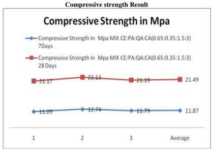
Cement 40% Replaced by Pond Ash and Sand 100% replaced by Quarry Dust
